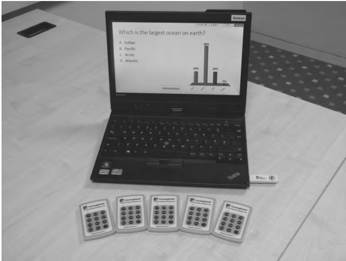
Figure 13.5: TurningPoint voting system. It comprises a receiver that is plugged into the USB port of a computer and a set of custom-built voting devices known as clickers.
